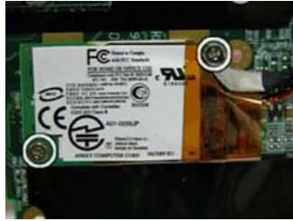
Fig. 33 Removing the MDC modem
